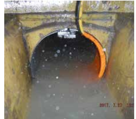
MSFM Area velocity flow meter installed downstream.
